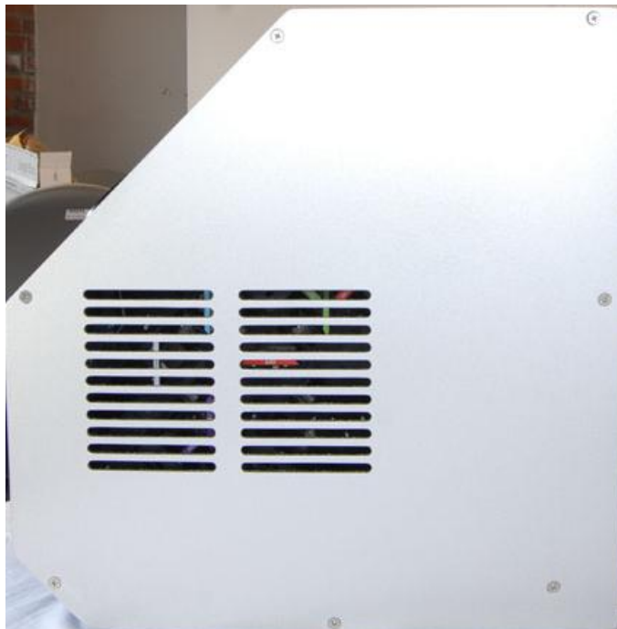
Figure 7 - Location of 7 panel screws
