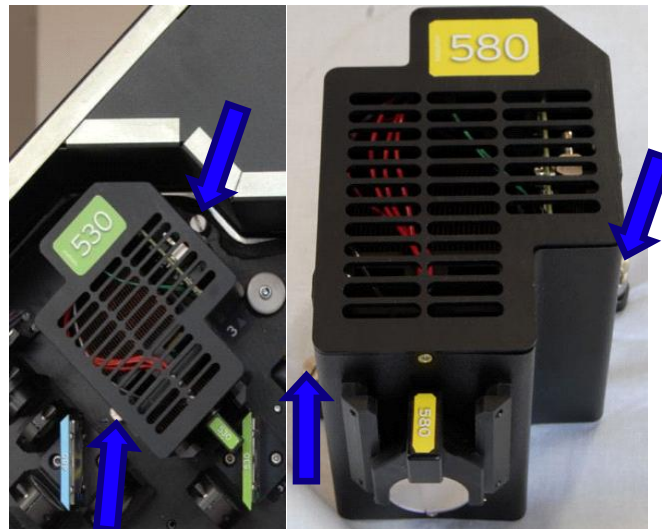
Figure 8 - Captive screws for module
